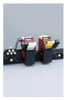
Because of the simultaneous marking of the cable start and cable end, great efficiency is obtained. The Z-284 is connected to a stripping machine. The existing interface allows the connection to products of different manufacturers.
